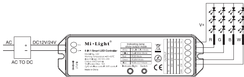
Controller connect to RGBW LED strip diagram
